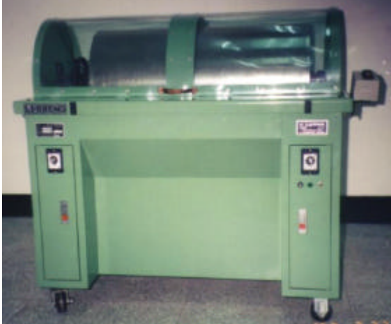
Clean the burrs out form capacitor core
